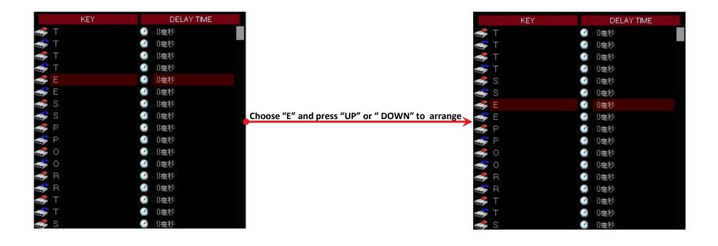
If you want to modify or insert Delay time and Key signal to the programmed macro, please click the INSERT button to modify the programmed macros.
